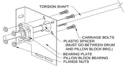
DUE TO THE LARGE SIZE OF THE OVERHEAD DOOR YOU HAVE PURCHASED PILLOW BLOCK BEARINGS HAVE BEEN SUPPLIED FOR ADDED STRENGTH AND SUPPORT. THE ABOVE DIAGRAM ILLUSTRATES THE INSTALLATION OF THE PILLOW BLOCK BEARING.
