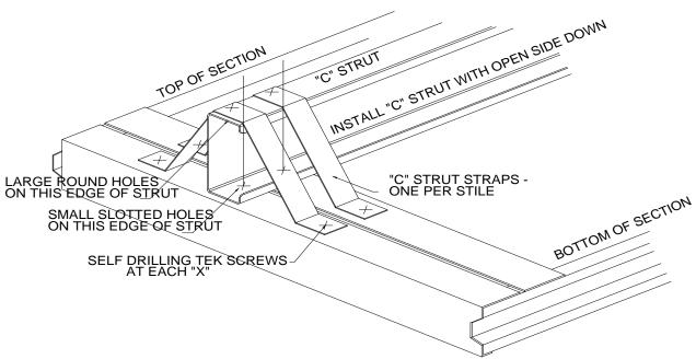
Special Note: When installing the "C" Strut on the top section of the door, first install the top corner brackets and then the "C" strut as close as possible to the top corner brackets.
